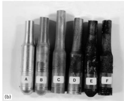
Figure 19 Changes in the degree of brightness of test bars solution heat-treated for 12 h at 510 °C followed by another 12 h at different temperatures (labelled A–F): (a) 0.06 wt % Mg, (b) ~0.5 wt % Mg. A, as-cast; B, 510 °C; C, 520 °C; D, 525 °C; E, 530 °C; F, 540 °C.
